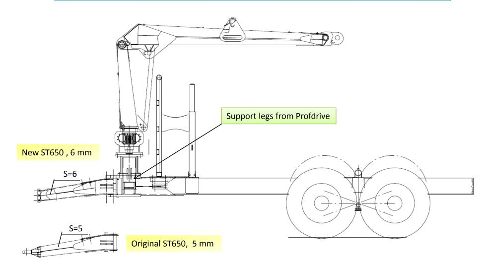
Draw bar thickness from 5 to 6 mm
